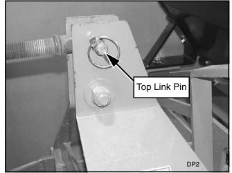
Figure 3. Top Link Attached to Aerator (Typical)
